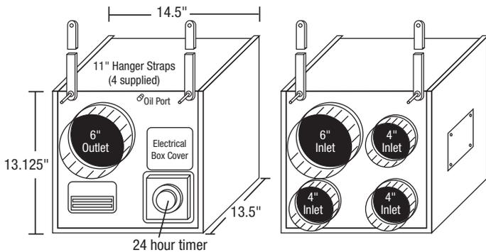
4" duct to the Ultra-Aire Quiet Vent (See Fig. 1). To make installation easy, the Ultra-Aire Quiet Vent has one 6" and three 4" duct inlet connections. The 6" outlet of the Ultra-Aire
